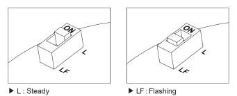
• Default function is set at steady LED. Select the desired function for your application during installation.
